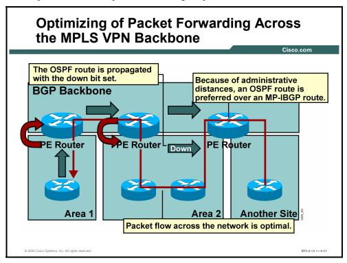
The OSPF superbackbone implementation with MP-BGP has other implications beyond the potential for routing loops between OSPF and BGP.
