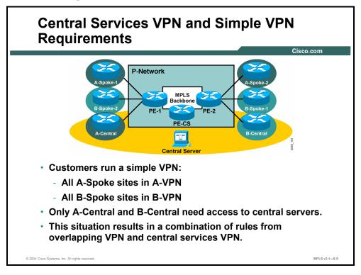
In this design, some of the customer sites need access to the central server. All other sites just need optimal intra-VPN access. The design is consequently a mixture of simple VPN topology and central services VPN topology.
