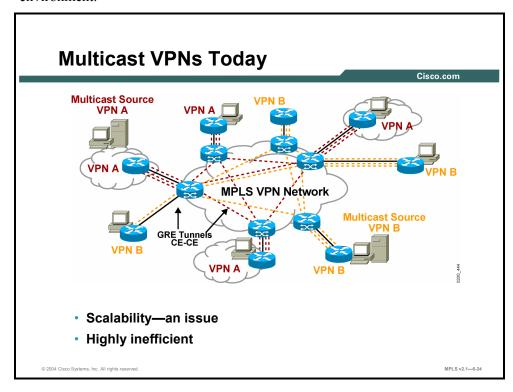
Historically, IPinIP generic routing encapsulation (GRE) tunnels were the only way to connect through a service provider network. Although such tunneled networks tend to have scalability issues, they represented the only means of passing IP multicast traffic through a VPN.
