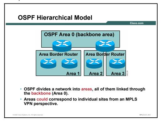
The OSPF routing protocol was designed to support hierarchical networks with a central backbone. The network running OSPF is divided into areas. All areas have to be directly connected to the backbone area (Area 0). The whole OSPF network (backbone area and any other connected areas) is called the OSPF domain.
