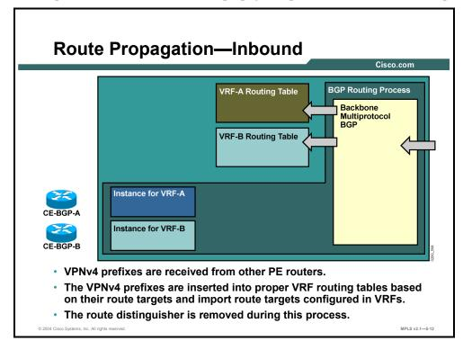
As other PE routers start originating VPNv4 routes, the MP-BGP process in the PE router here receives the routes. The routes are filtered based on RT attributes attached to them, and are inserted into the proper per-VRF IP routing tables based on the import RTs configured for individual VRFs. The RD that was prepended by the originating PE router is removed before the route is inserted into the per-VRF IP routing table.
