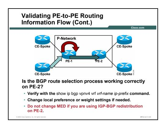
In complex environments with multihomed customer sites, the BGP route selection process might affect proper MPLS VPN operation. Use standard BGP route selection tools (weights or local preference) to influence BGP route selection. The MED attribute should not be changed inside the MPLS VPN backbone if you plan to use two-way route redistribution between the PE-CE routing protocol and BGP.
