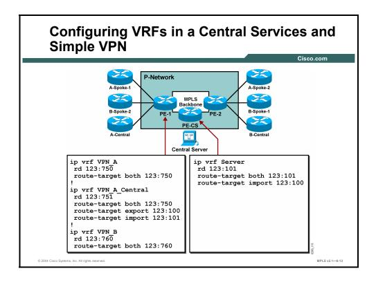
Use the **ip vrf** command to configure VRFs in a central services and simple VPN.
