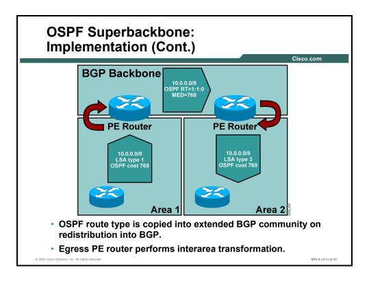
This figure illustrates the propagation of internal OSPF routes across the MPLS VPN superbackbone.
