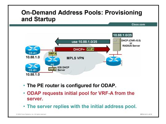
As soon as the DHCP server is enabled on the PE router that has ODAP enabled, the PE router will request an initial address pool from its designated server.
