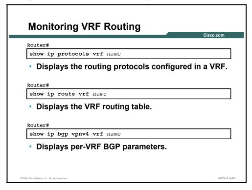
The following three commands can be used to monitor VRF routing:
