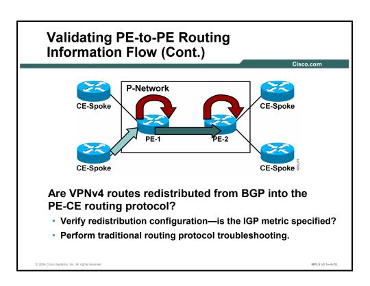
Finally, the BGP routes received via MP-BGP and inserted into the VRF need to be redistributed into the PE-CE routing protocol. A number of common redistribution mistakes can occur here, starting with missing redistribution metrics.
