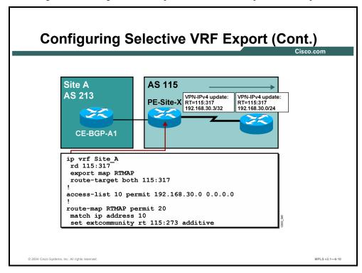
In the earlier example, selective import of routes into a VRF was achieved with an import route map in the receiving VRF that allowed only routes from a certain address block to be inserted into the VRF. In this example, routes from a certain address block are marked with an additional RT in the originating VRF and are automatically inserted into the receiving VRF on the basis of their RT.
