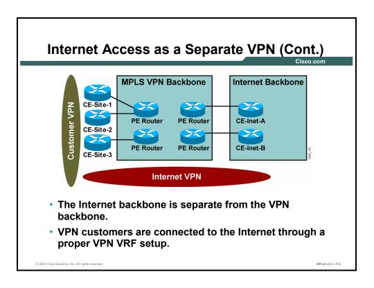
When you implement Internet access as a separate VPN, the Internet backbone is kept separate from the MPLS VPN backbone—resulting in increased security for the MPLS VPN backbone (for example, Internet hosts can reach only PE routers, but not the provider routers [P routers]). The VPN customers are connected to the Internet simply through proper VRF setup.
