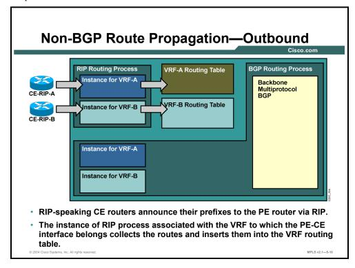
RIP-speaking CE routers identify the correct instance of RIP on the PE router when an inbound PE interface is associated with a VRF. This association allows CE routers to announce their networks to the appropriate per-VRF routing table.
