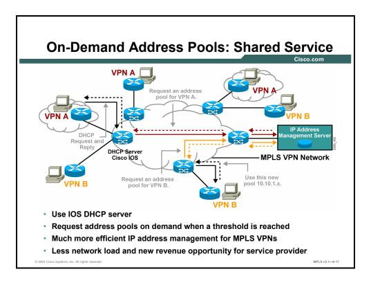
With MPLS VPNs, service providers have to allocate their IP address pools to independent RADIUS or DHCP servers for each VPN. Once the site threshold has been reached, new addresses have to be provided manually. With ODAP for MPLS VPNs, this process can now be fully automated and provided as a shared service on one or more servers. When the site threshold is exceeded, ODAP automates the process of expanding the overall address pool, reducing network loading and performing configuration.
