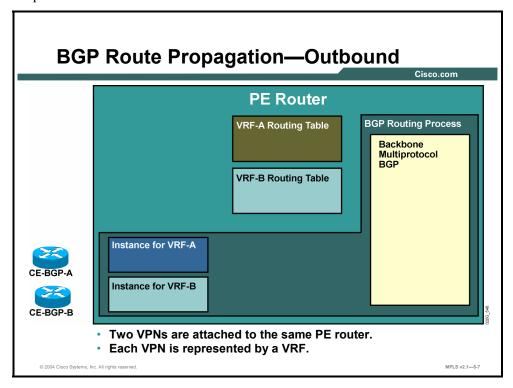
This figure and the following figures illustrate the interactions between VRF instances of routing processes, VRF routing tables, and the global VPNv4 BGP routing process.
