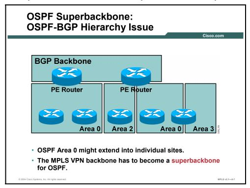
The MPLS VPN architecture extends the OSPF architecture by introducing another backbone above OSPF Area 0, the superbackbone. The OSPF superbackbone is implemented with MP-BGP between the PE routers but is otherwise completely transparent to the OSPF routers. The architecture even allows disjointed OSPF backbone areas (Area 0) at MPLS VPN customer sites.
