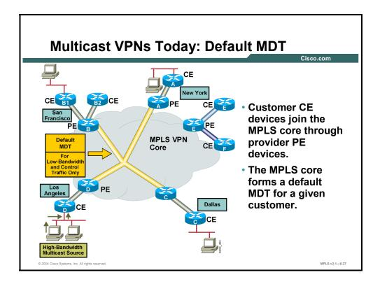
Multicast VPNs establish a static default multicast distribution tree (MDT) for each multicast domain. The default MDT defines the path used by PE routers to send multicast data and control messages to every other PE router in the multicast domain.
