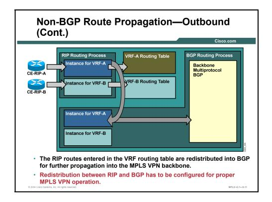
MP-BGP is used in the MPLS VPN backbone to carry VPN routes (prefixed with the RD) as 96-bit VPNv4 routes between the PE routers. The backbone BGP process looks exactly like a standard Internal Border Gateway Protocol (IBGP) setup from the perspective of the VRF. The per-VRF RIP routes therefore *must be redistributed* into the per-VRF instance of the BGP process to allow them to be propagated through the backbone MP-BGP process to other PE routers.
