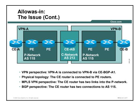
The setup in which a customer router links two VPNs in an MPLS VPN backbone can be viewed from several different perspectives, as follows:
