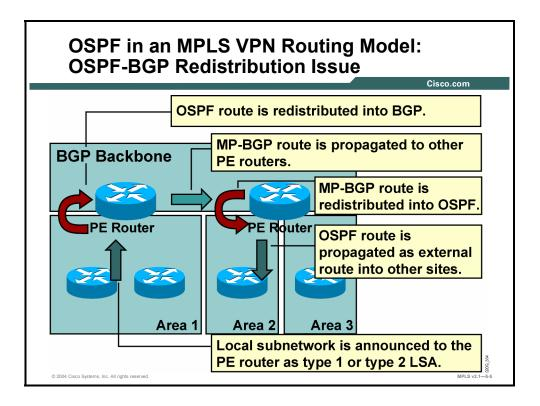
The IGP-BGP redistribution introduced by the MPLS VPN routing model does not fit well into customer networks running OSPF. When an OSPF customer is migrated to an MPLS VPN service, any route that is redistributed into OSPF from another routing protocol will now be redistributed as an external OSPF route. The OSPF routes received by one PE router are propagated across the MPLS backbone and redistributed back into OSPF at another site as external OSPF routes.
