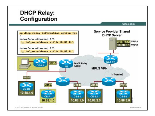
The **dhcp relay information option vpn** command enables the system to insert VPN suboptions into the DHCP relay agent information option in forwarded BOOTREQUEST messages to a DHCP server and sets the gateway address to the outgoing interface toward the DHCP server. The VPN suboptions are also added to the BOOTP broadcast packets when the command is configured.
