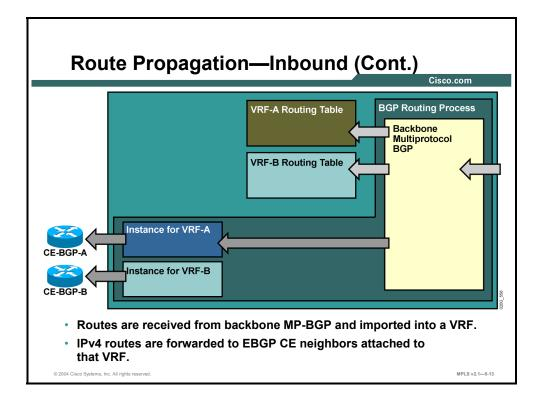
The Multiprotocol Internal Border Gateway Protocol (MP-IBGP) VPNv4 routes received from other PE routers and selected by the import RTs of a VRF are automatically propagated as 32-bit IPv4 routes to all BGP-speaking CE neighbors of the PE router.
