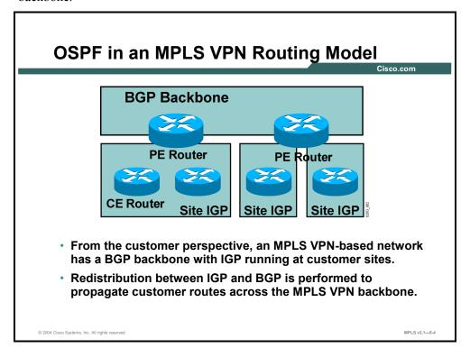
The MPLS VPN routing model introduces a BGP backbone into the customer network. Isolated copies of IGP run at every site, and MP-BGP is used to propagate routes between sites. Redistribution between customer IGP—running between PE routers and CE routers—and the backbone MP-BGP, is performed at every PE router.
