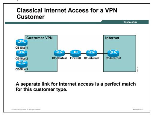
The classical Internet access setup for a VPN customer is based on a separated Internet access design model. This design model is thus a perfect match for customers looking for classical Internet access service.
