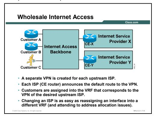
Wholesale Internet access is implemented by creating a separate VPN for every upstream ISP. The Internet gateway of the upstream ISP (acting as a CE router toward the MPLS VPN-based Internet access backbone) announces a default route, which is used for routing inside the VPN.
