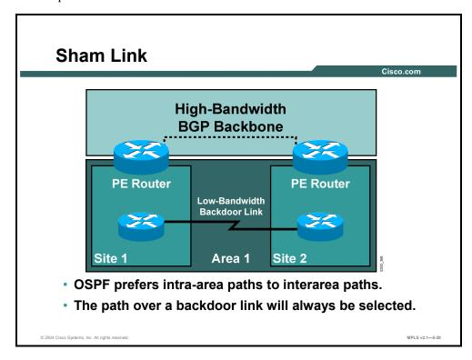
Although OSPF PE-CE connections assume that the only path between two client sites is across the MPLS VPN backbone, backdoor paths between VPN sites may exist.
