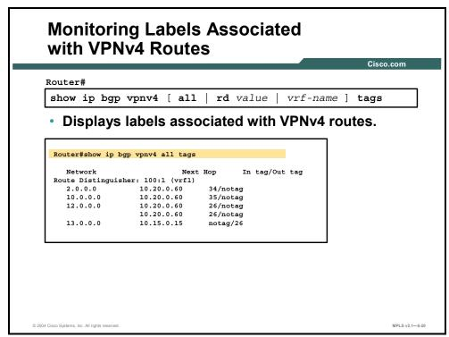
You can use the **show ip bgp vpnv4 tags** command to display tags assigned to local or remote VRF routes by the local or remote PE router. This command displays tags associated with all VPNv4 routes when you use the all keyword. This command can also display tags associated with a specified RD or VRF.
