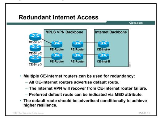
Redundant Internet access is easy to achieve when the Internet service is implemented as a VPN in the MPLS VPN backbone, as described here:
