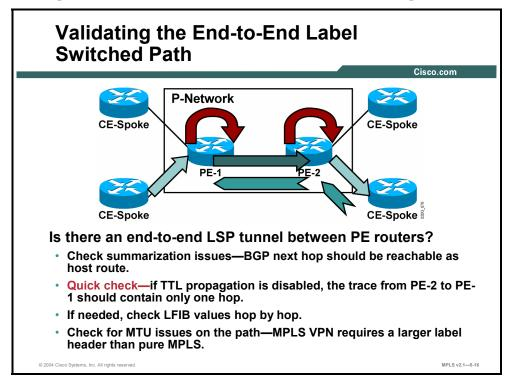
If CEF is enabled on the ingress interface and the CEF entry contains proper labels, the data flow problem might lie inside the MPLS core. Two common mistakes include summarization of BGP next hops inside the core IGP and MTU issues.
