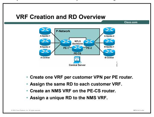
The VRF and RD design is the same as with central services VPNs. The only difference between this topology and the central services VPN topology combined with a simple VPN topology is the RT marking process during route export.
