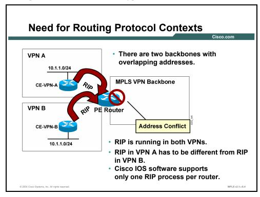
Traditional Cisco IOS software can support a number of different routing protocols. In some cases, even several completely isolated copies of the same routing protocol are supported. For example, several Open Shortest Path First (OSPF) processes can be used.
