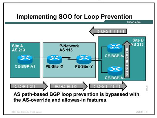
Most aspects of BGP loop prevention are bypassed when either the AS-override feature or the allowas-in feature is used. The routing information loops can still be detected by manually counting occurrences of an AS number in the AS path in an end-to-end BGP routing scenario then ensuring that the number field in the **neighbor allowas-in** command is set low enough to prevent loops.
