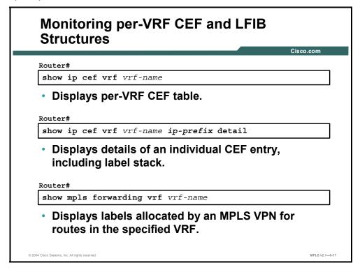
The following three commands can be used to display per-VRF FIB and LFIB structures:
