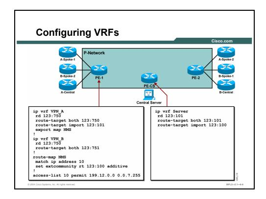
You can have a configuration for a customer VRF with differentiated RT export for loopback addresses.
