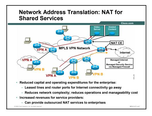
The integration of NAT with MPLS VPNs allows multiple MPLS VPNs to be configured on a single device to work together. NAT can differentiate from which MPLS VPN that it receives IP traffic, even if the MPLS VPNs are all using the same IP addressing scheme. This enhancement enables multiple MPLS VPN customers to share services while ensuring that each MPLS VPN is completely separate from the other.
