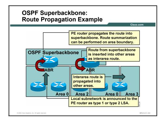
The MPLS VPN superbackbone appears as another layer of hierarchy in the OSPF architecture. The PE routers that connect regular OSPF areas to the superbackbone therefore appear as OSPF Area Border Routers (ABRs) in the OSPF areas to which they are attached. In Cisco IOS implementation, ABRs also appear as Autonomous System Boundary Routers (ASBRs) in nonstub areas.
