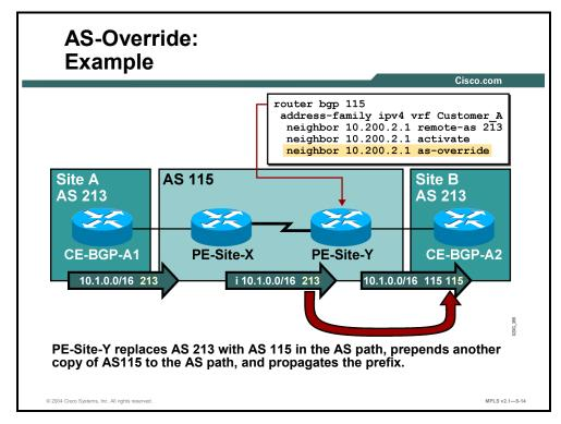
The AS-override mechanism, configured on the PE-Site-Y router, replaces the customer AS number (213) with the provider AS number (115) before sending the update to the customer site. An extra copy of the provider AS number is prepended to the AS path during the standard EBGP update process.
