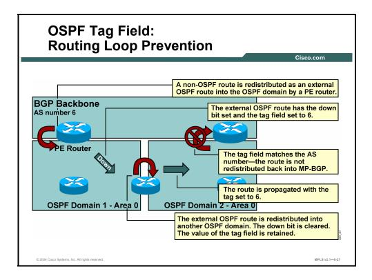
The OSPF tag field can be used to prevent routing loops when the redistribution is done between OSPF domains.
