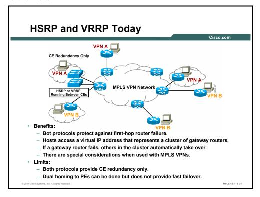
Today, service providers face challenges when it comes to implementing an efficient redundancy scheme. To address many of these issues, Cisco has offered HSRP and VRRP, which have provided the following benefits:
