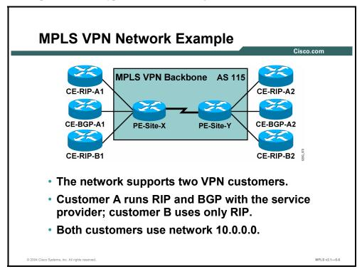
To illustrate the use of MPLS VPN configuration commands, you can look at a configuration of the PE router in a sample network.
