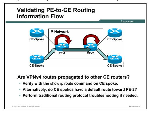
Last but not least, the routes redistributed into the PE-CE routing protocol have to be propagated to CE routers. You may also configure the CE routers with a default route toward the PE routers (see note). Use standard routing protocol troubleshooting techniques in this step.
