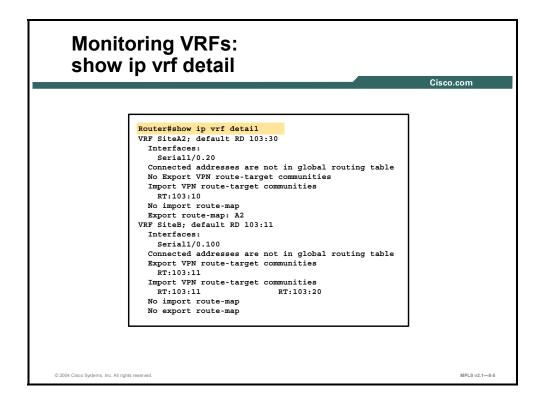
To display detailed information on the VRFs and associated interfaces, use the **show ip vrf detail** command. This table describes the additional fields shown by this command.
