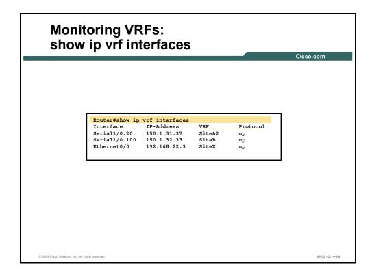
To display the interfaces bound to a particular VRF (or interfaces bound to any VRF), use the show ip vrf interfaces command, which displays the fields described in this table.
