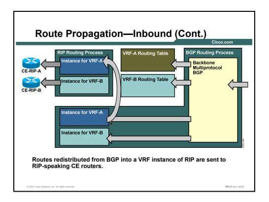
When the IBGP routes from the per-VRF IP routing table are successfully redistributed into the per-VRF instance of the RIP process, the RIP process announces these routes to RIP-speaking CE routers, thus achieving transparent end-to-end connectivity between the CE routers.
