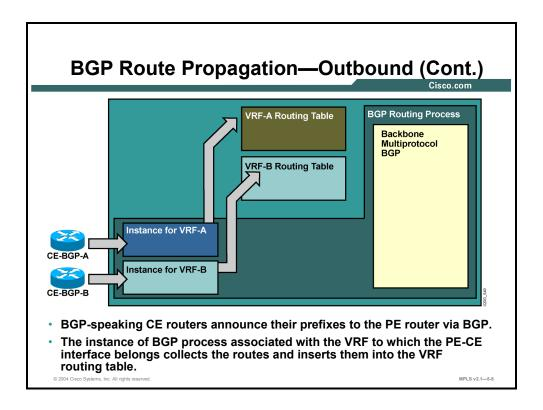
The BGP-speaking CE routers announce their networks via EBGP sessions to the PE router. The CE routers are BGP neighbors of the PE router. The PE router associates each BGP neighbor relationship with individual VRFs that enable the various instances of the BGP routing process to put the received routing updates into the proper per-VRF routing table.
