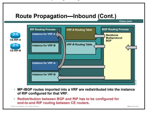
The MP-IBGP routes, although they are inserted in the per-VRF IP routing table, are *not* propagated to RIP-speaking CE routers automatically. To propagate these MP-IBGP routes to the RIP-speaking CE routers, you must manually configure the redistribution between per-VRF instance of BGP and per-VRF instance of RIP.
