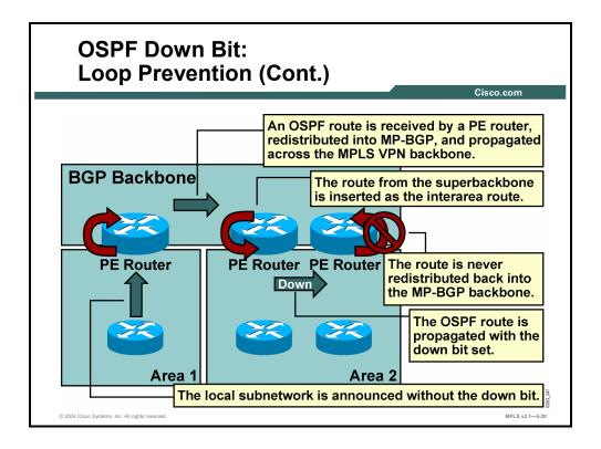
The down bit is used between the PE routers to indicate which routes were inserted into the OSPF topology database from the MPLS VPN superbackbone and thus shall not be redistributed back in the MPLS VPN superbackbone. The PE router that redistributes the MP-BGP route as an OSPF route into the OSPF topology database sets the down bit. The other PE routers use the down bit to prevent this route from being redistributed back into MP-BGP.
