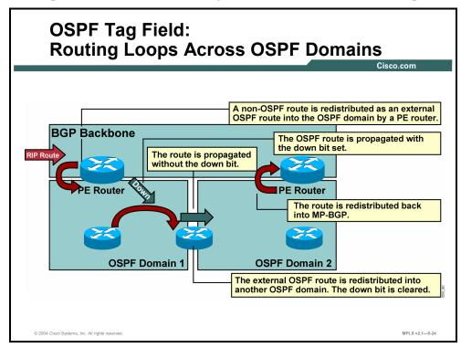
The down bit stops the routing loops between MP-BGP and OSPF. The down bit cannot, however, stop the routing loops when redistribution between multiple OSPF domains is involved.
