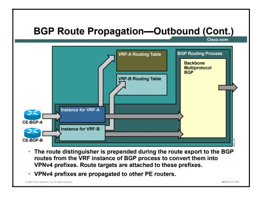
This figure illustrates the interactions between VRF instances of routing processes, VRF routing tables, and the global VPNv4 BGP routing process.
