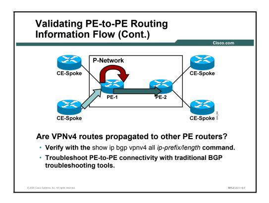
The CE routes redistributed into MP-BGP need to be propagated to other PE routers. Verify proper route propagation with the **show ip bgp vpnv4 all** *ip-prefix* command on the remote PE router.
