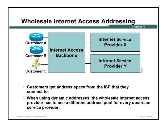
Regardless of the business model used in the wholesale Internet access service, the addressing requirements are always the same: the upstream ISP allocates a portion of its address space to the end users connected to the Internet access backbone. The wholesale Internet access provider consequently has to use a different address pool for every upstream ISP.
