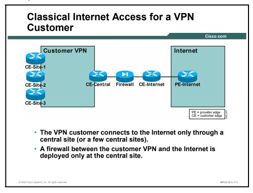
Classical Internet access is implemented through a (usually central) firewall that connects the customer network to the Internet in a secure fashion. The private network of the customer (or VPN if the customer is using a VPN service) and the Internet are connected only through the firewall.
