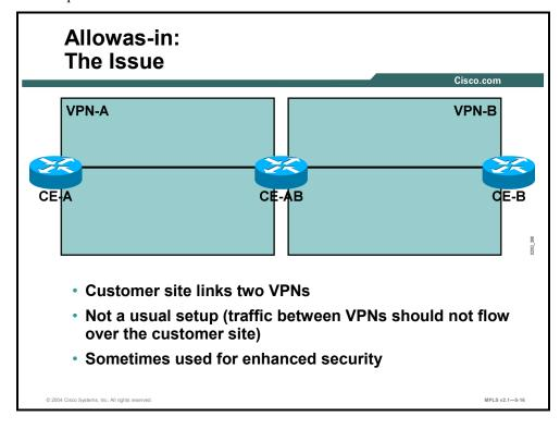
In some security-conscious implementations, customer VPNs are linked by a customer router that performs security functions, such as access filtering or access logging.
