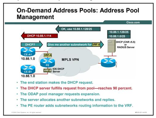
The PE router will honor DHCP requests and assign addresses until its address pool is 90 percent depleted. At this point, the PE router will request an extension of the address pool from its designated server.
