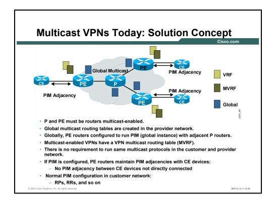
For every multicast domain of which an MVRF is a part, the PE router creates a multicast tunnel interface. A multicast tunnel interface is an interface that the MVRF uses to access the multicast domain. It can be thought of as a conduit that connects an MVRF and the global MVRF. One tunnel interface is created per MVRF.
