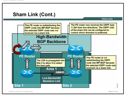
Because the sham link is seen as an intra-area link between PE routers, an OSPF adjacency is created and database exchange (for the particular OSPF process) occurs across the link. The PE router can then flood LSAs between sites from across the MPLS VPN backbone. As a result, the desired intra-area connectivity is created.
