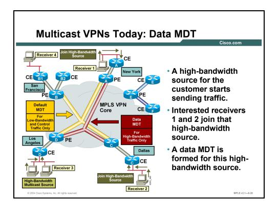
Multicast VPNs also support the dynamic creation of MDTs for high-bandwidth transmission. Data MDTs are a feature unique to Cisco IOS software. Data MDTs are intended for high-bandwidth sources, such as full-motion video inside the VPN, to ensure optimal traffic forwarding in the MPLS VPN core. The threshold at which the data MDT is created can be configured on a per-router or a per-VRF basis.
