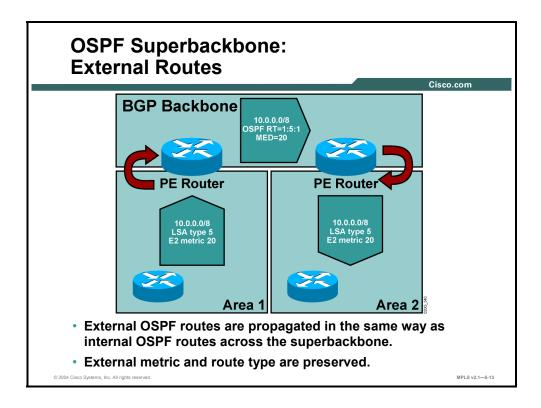
The external OSPF routes are redistributed into MP-BGP in exactly the same way as the internal OSPF routes. The following describes how the process changes slightly on the receiving PE router:
