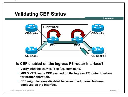
One of the most common configuration mistakes related to data flow is the failure to enable CEF in the ingress PE router interface. The presence of CEF can be verified with the **show cef interface** command. CEF is the only switching method that can perform per-VRF lookup and thus support MPLS VPN architecture.
