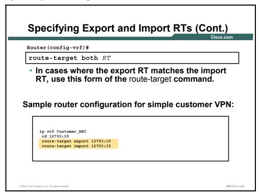
Whenever an RT is both an import and an export RT for a VRF, you can use the **route-target** both command to simplify the configuration. For example, the two "route-target" configuration lines in the sample router configuration in the figure could be reduced to a single command: route-target both 12703:15.
