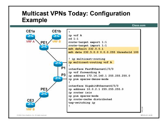
Configuring VPN-aware multicast capability is a combination of standard VPN, standard multicast, and new VPN-aware multicast commands.
