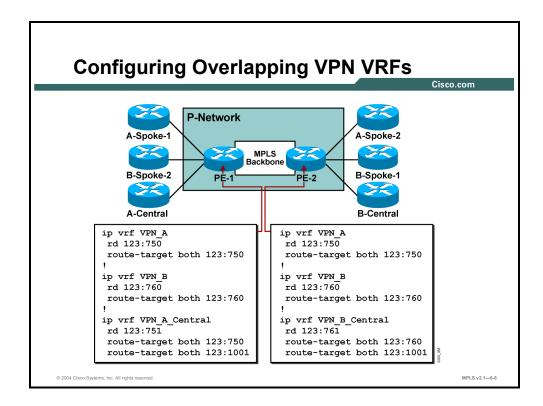
The Cisco IOS software configuration for PE-1 and PE-2 reflects the RT and RD numbering scheme from the two tables.
