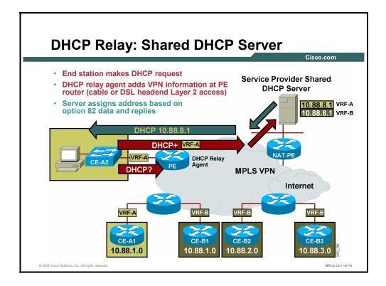
Typical network topology for a shared DHCP server involves a bridged access to the remote location via DSL or cable modem technology. Aggregation into the PE router involves the use of headend equipment, such as digital subscriber line access multiplexer (DSLAM) and cable modem termination system (CMTS).
