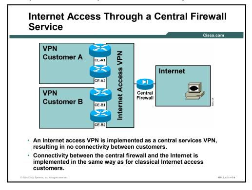
The central managed firewall service should be implemented with the central services VPN topology—with the central firewall being the server site and all customer CE routers residing in client sites. For customers with their own VPNs implemented over the same MPLS VPN backbone, the topology that overlaps customer VPN and central services VPN should be used.
