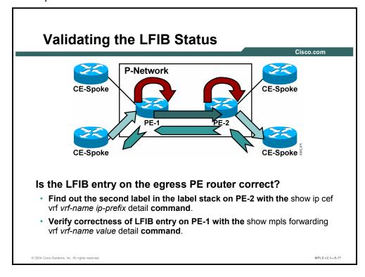
As a last troubleshooting measure (usually not needed), you can verify the contents of the LFIB on the egress PE router and compare them with the second label in the label stack on the ingress PE router. A mismatch indicates an internal Cisco IOS software error that you will need to report to the Cisco Technical Assistance Center (TAC).
