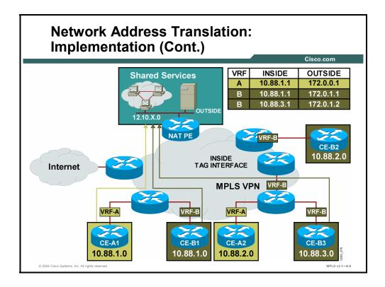
There are two approaches to implementing NAT in the MPLS VPN network. NAT can be implemented on the CE router, which is already supported by NAT, or it can be implemented on a PE router. Integration of NAT with MPLS VPNs enables the implementation of NAT on a PE router in an MPLS cloud.
