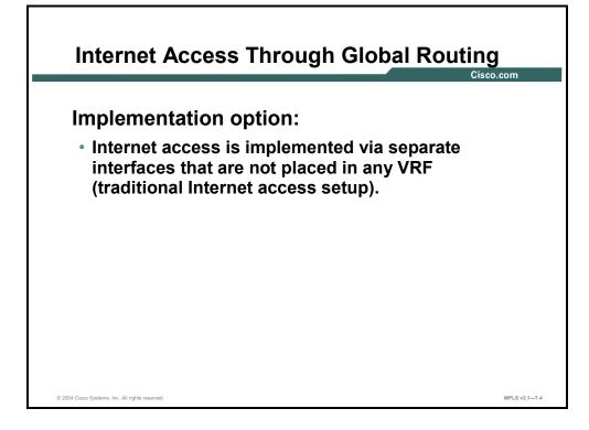
Implementing Internet access through global routing is identical to building an IP backbone offering Internet services. IP version 4 (IPv4) Border Gateway Protocol (BGP) is deployed between the PE routers to exchange Internet routes, and the global routing table on the PE routers is used to forward the traffic toward Internet destinations.
