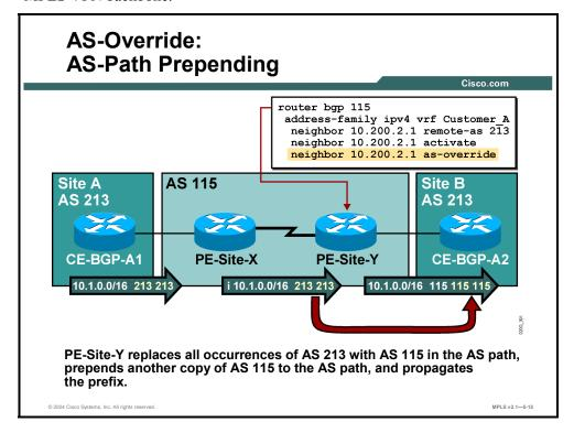
The PE router has to send a route with an AS path containing multiple copies of the customer AS number to the CE router. In this case, all the leading copies of the customer AS number are replaced with the provider AS number (resulting in two occurrences of the provider AS number in the example), and the third occurrence of the provider AS number is prepended to the BGP update before it is sent to the CE router.
