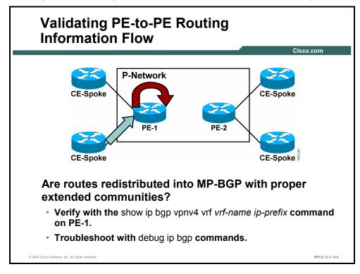
The CE routes received by the PE router need to be redistributed into MP-BGP; otherwise, they will not get propagated to other PE routers. Common configuration mistakes in this step include the following:
