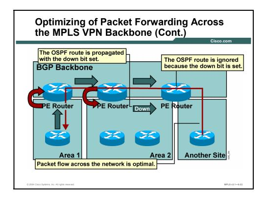
With the new route OSPF selection rules in place, the packet forwarding in the network shown in the figure follows the desired path. The process steps are described in this table.
