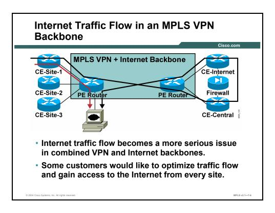
The traffic flow issue becomes even more pronounced when the customer VPN (based on, for example, MPLS VPN services) and the Internet traffic share the same service provider backbone. In this case, the traffic from a customer site may have to traverse the service provider backbone as VPN traffic and then return into the same backbone by the corporate firewall, ending up at a server very close to the original site.
