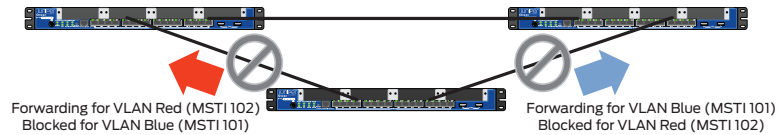
Figure 8: Multiple Spanning Tree Protocol
